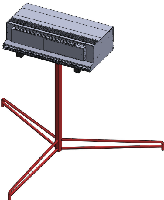
Ensure fixture is properly supported and resting on the metalwork and not the fragile glass parts. Do not remove blue protective film at this stage.
