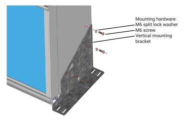
Attach the vertical mounting brackets with the 6x M6x16mm bolts and anti-vibration washers.
