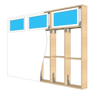
Prepare a wall with sufficient strength to support the fixtures (refer to Spec Sheets for dimensions and weights). It is recommended to locate the fixture above eye level for a more convincing viewing experience.
