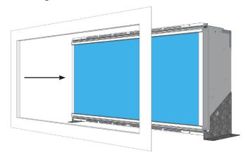
Once the drywall has been finished. Using a long nose (needle nose) plier. Grab one of the four aircrft wires hanging from the fixture and pull it outwards and slot into the slots on the Bezel Trim. The wires are spring loaded and will pull up the trim.
